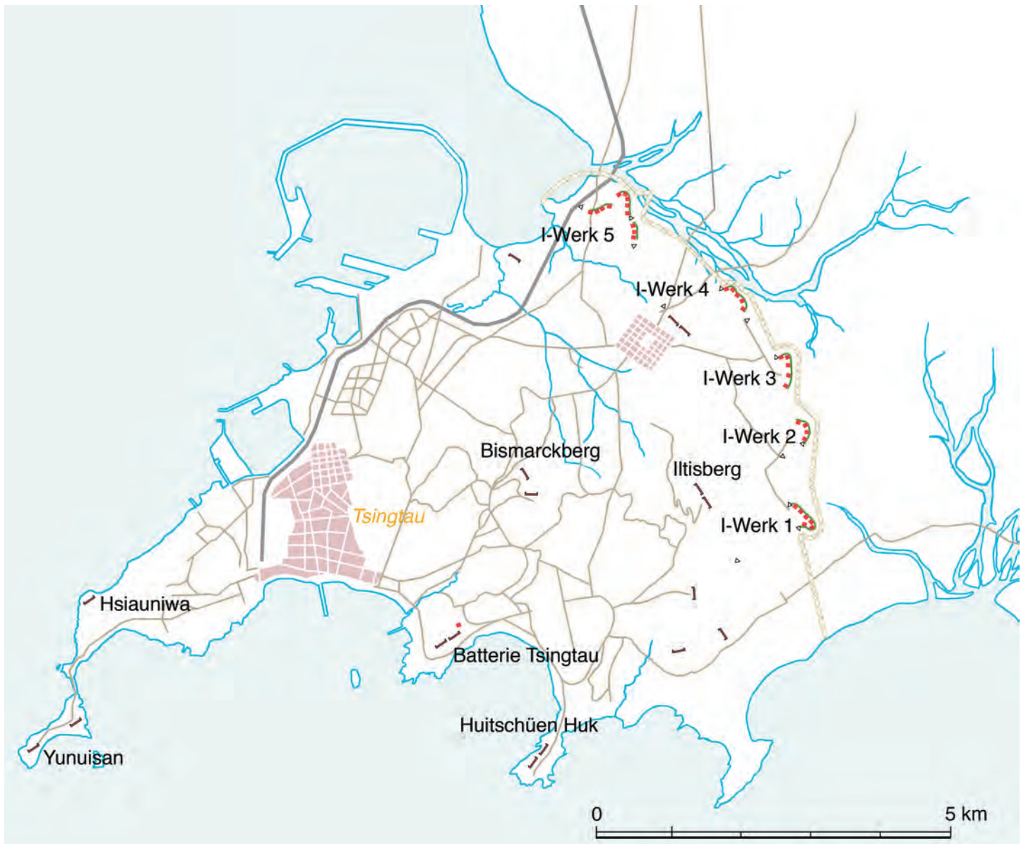
The German protectorate of Tsingtau in China was fortified from 1902 onward. The landfront in the east was defended by five infantry works with a series of field gun batteries and machine gun positions. The southern seafront was provided with naval batteries along the shore, while on the central Bismarckberg a 28-cm howitzer battery commanded the peninsula and its surrounding waters.
